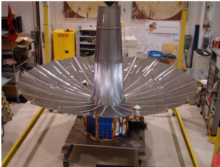
**Figure 2: Deployed TacSat-4 UHF Reflector on Comm-X Payload**
