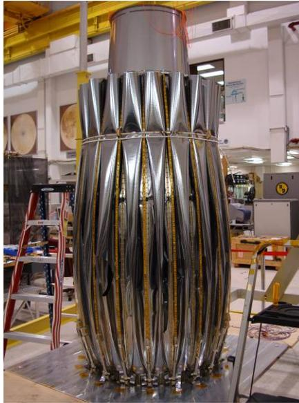
**Figure 1: Stowed TacSat-4 UHF Antenna**
