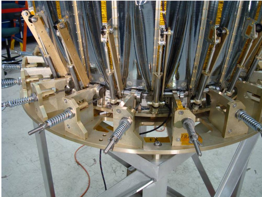
**Figure 7: Gravity Offloading Fixture**
