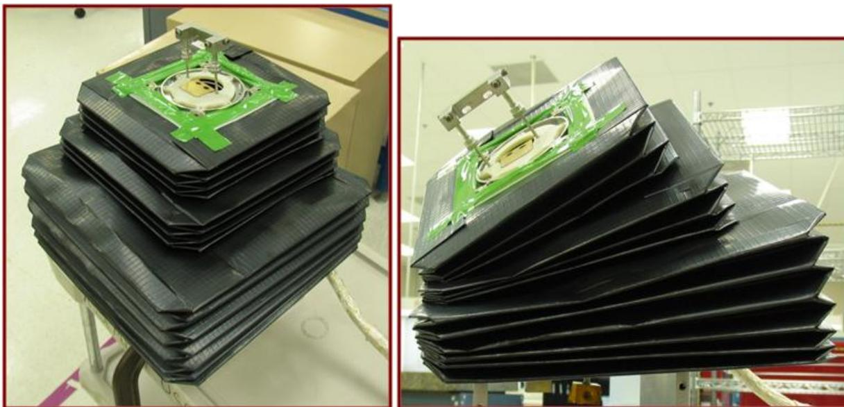
Figure 8. Multilayer Insulation (MLI) Blanket
