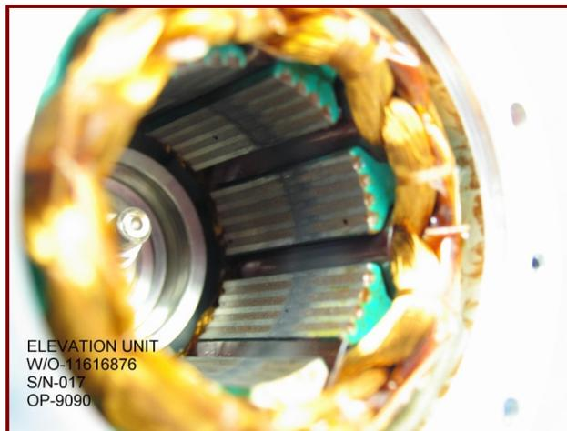
**Figure 10. Stator**
