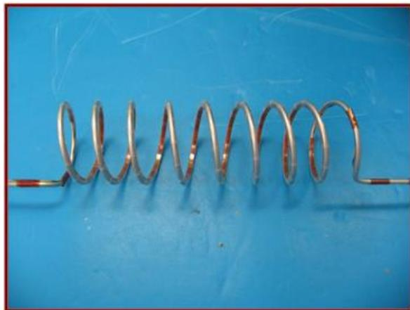
Figure 5. Inner Propellant Tubing with Heater
