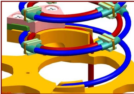
Figure 6. Propellant Line Assembly with Spacers
