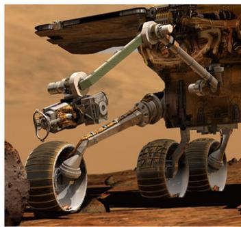
**Figure 1 Mars Exploration Rover Instrumentation Deployment Device.**
