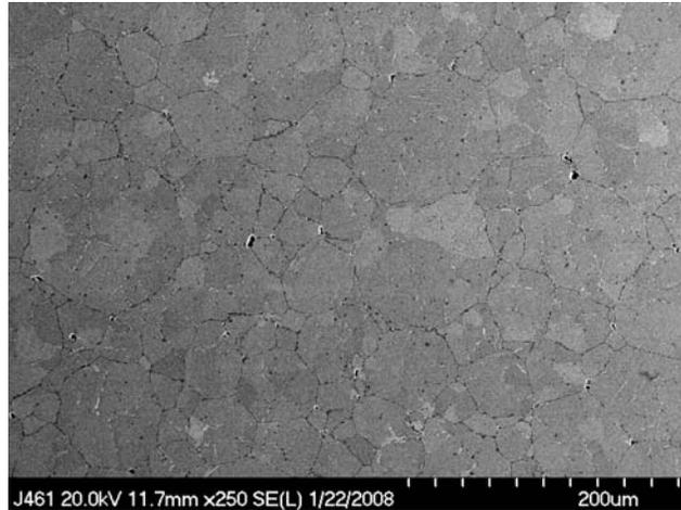
**Figure 2. Cross-section electron micrograph of Nitinol 60 ball.**
