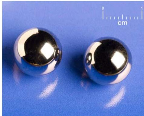
Figure 1. Nitinol 60 grade 5 test balls.
