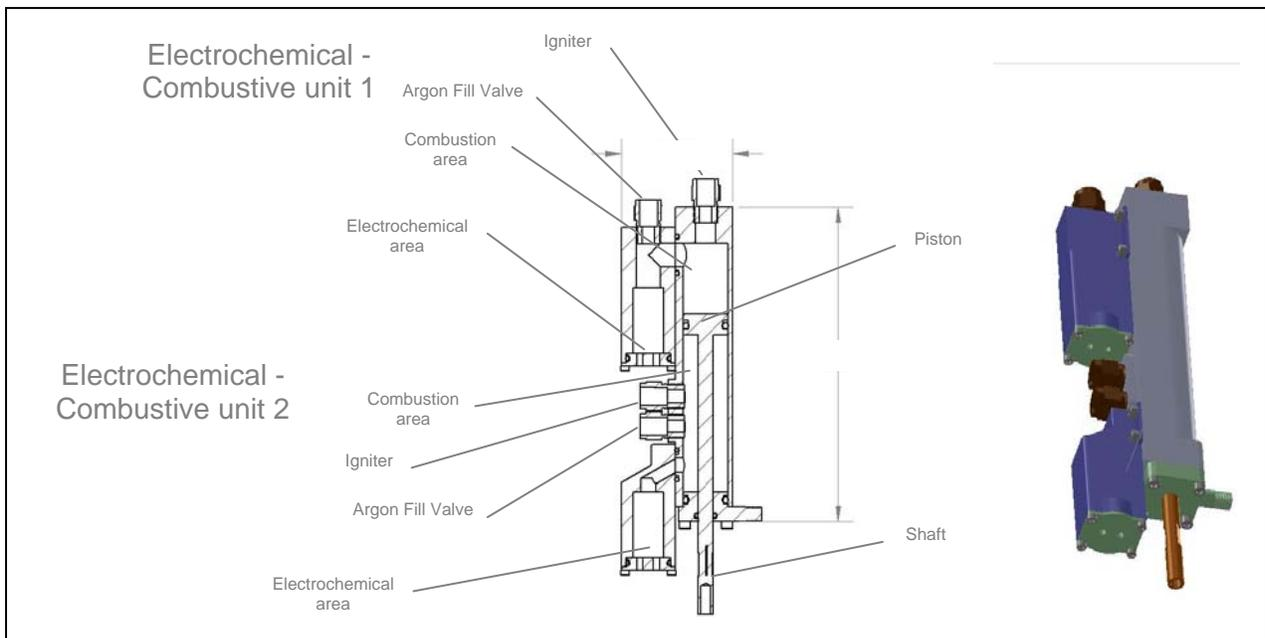
**Figure 12. Bidirectional Actuator for the Rotor Blade Application**
