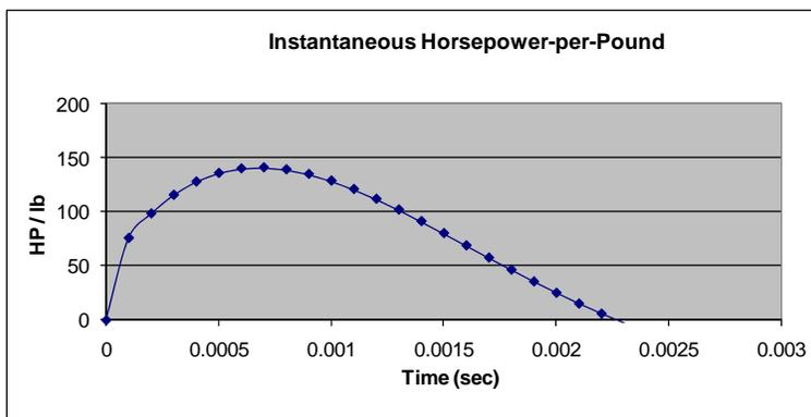
**Figure 11. Specific Power Throughout Test Fixture Stroke**
