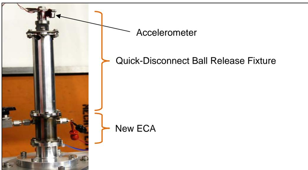
**Figure 7. Complete Peak Power Density Test Fixture**
