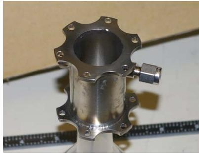
**Figure 5. Lightweight Electrolysis Combustion Actuator (ECA)**
