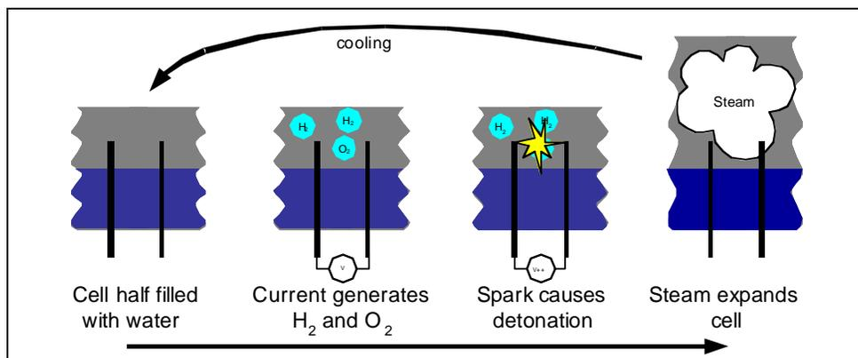
**Figure 2. Schematic Drawing of the Actuation Cycle**
