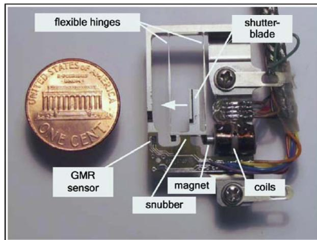
**Figure 1: Complete integrated shutter mechanism with milled titanium structure (EM, Engineering Model). The arrow near the shutter-blade indicates the displacement direction for the 1.5-mm movement.**
