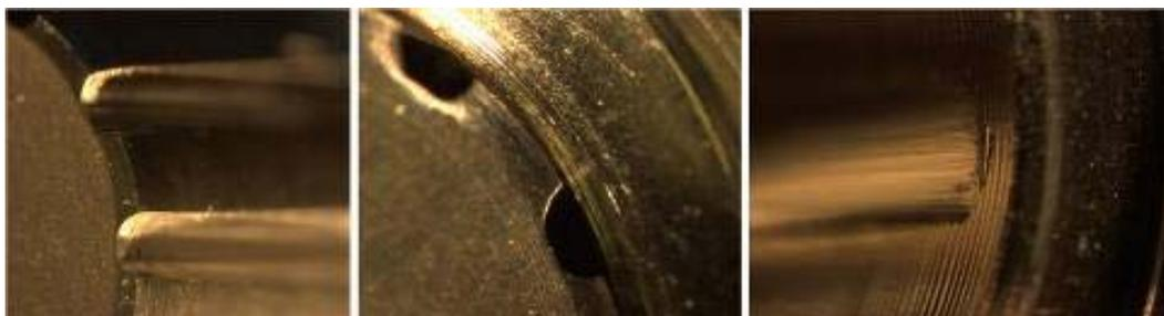
**Figure 17: Passed pressing trial results with 40 μm oversize**
