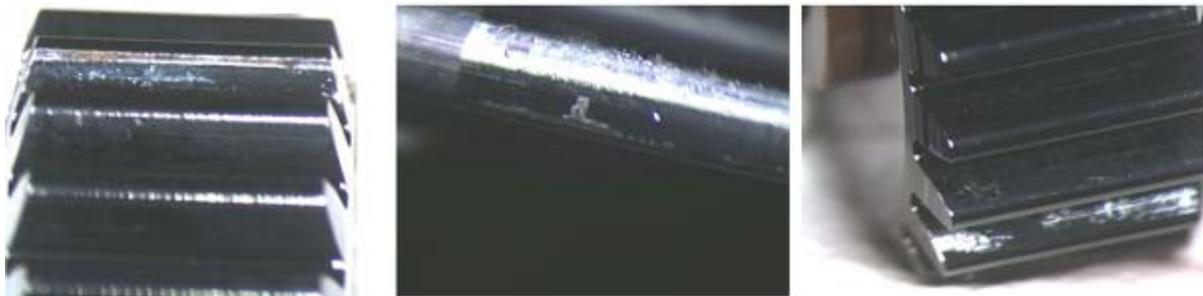
**Figure 19: Coating damage after vibration**
