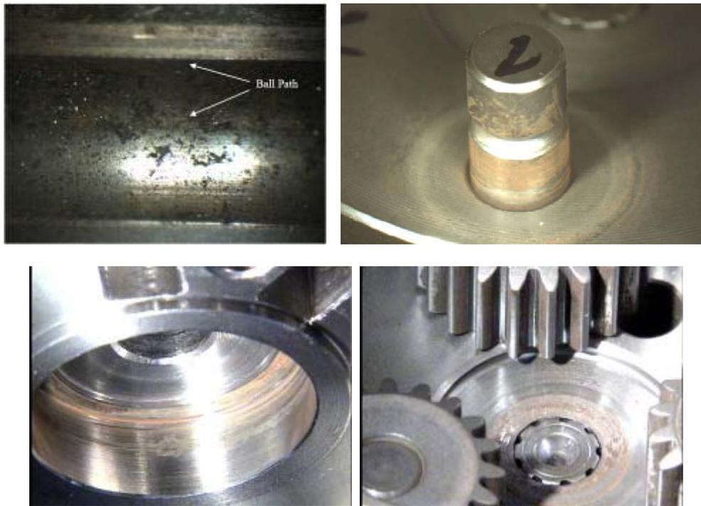
**Figure 3: Lubrication failure of first actuator after life test<sup>1</sup>**
