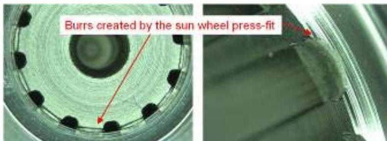
**Figure 16: Failed pressing trial results**
