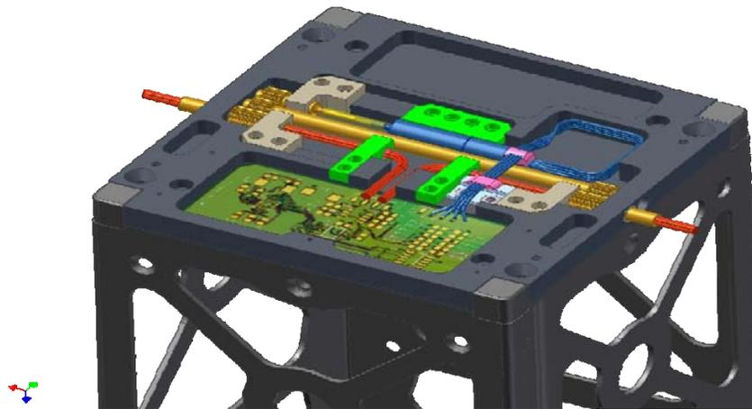
**Figure 5: Inner workings of the prototype SADA shown on typical CubeSat structure. The drive fits into the typically unused space at the end of a standard frame (e.g. Pumpkin<sup>V</sup>).**
