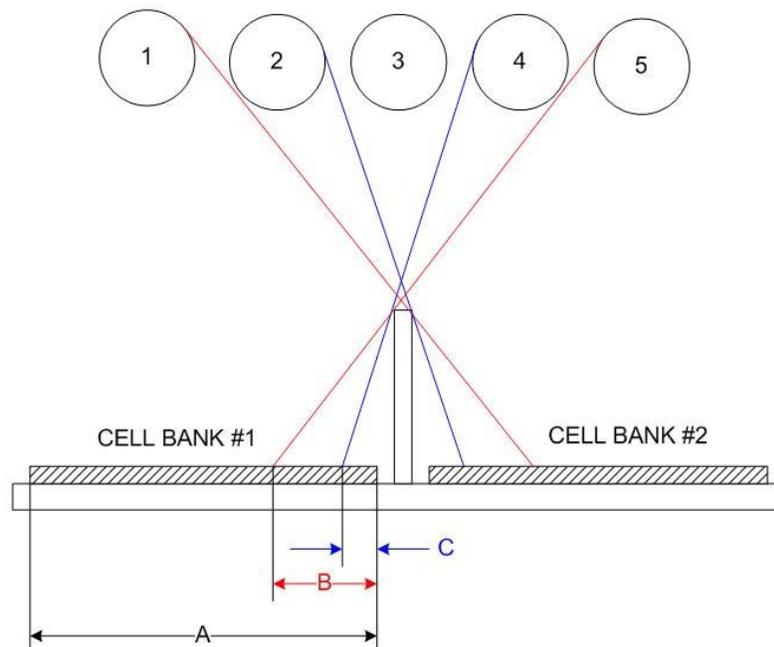
**Figure 6: Illustration of Sun angle to obscured portion of cell banks. Note that of the total available area (represented by ‘A’) the obscured area (‘B’ and ‘C’) decreases as the light source becomes normal to the panel surface. By comparing the output of the two banks shown, we are able to determine gross array position relative to the Sun.**
