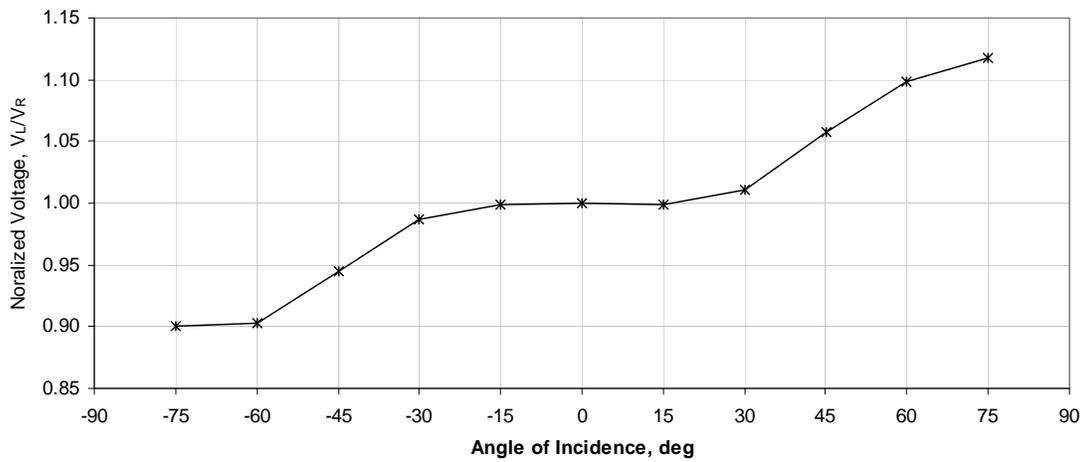
**Figure 8: Characterization of breadboard solar array configuration with raised, intra-bank barrier. The top graph shows the output of the individual strings as a function of Sun (gimbal) position; the bottom graph shows the normalized voltage ratio.**
