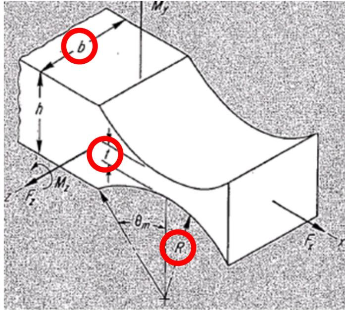
Figure 3. Flexure dimensions [2]
