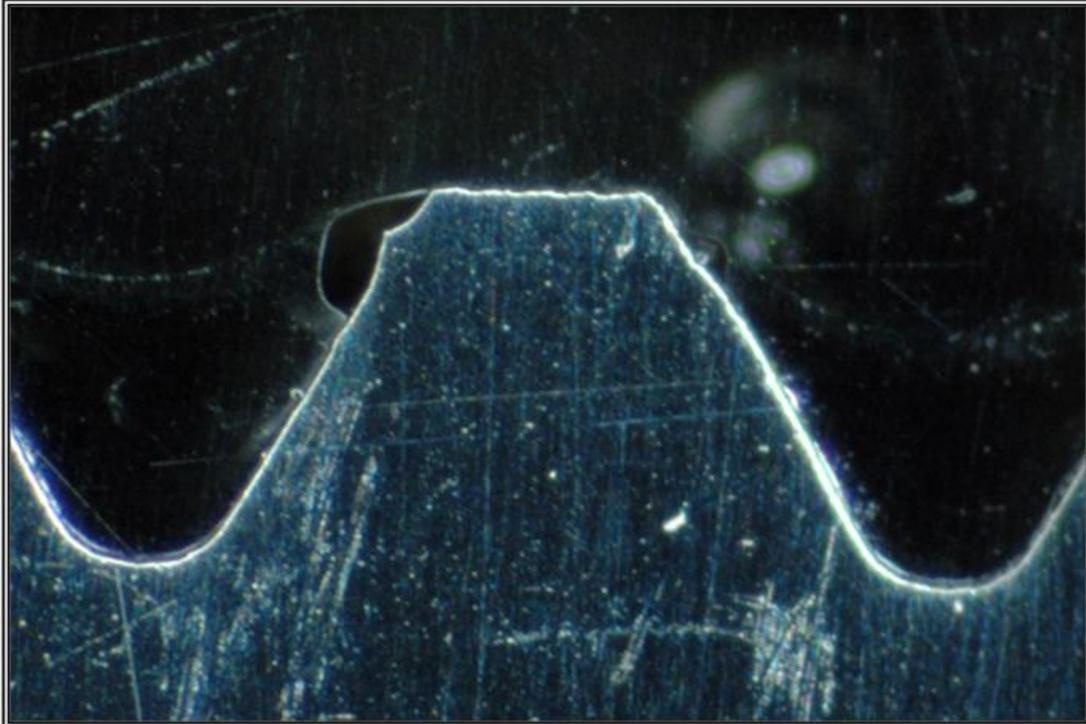
**Figure 2: Surface Finish error, burr; 500x magnification**
