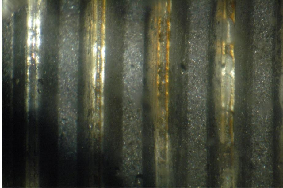
**Figure 6: Amber coloration of resin binder; 50x magnification**
