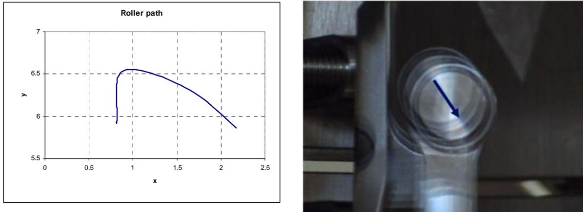
**Figure 3 Theoretical (left) versus measured (right) trajectory of the Latch onto the Latch Tab**
