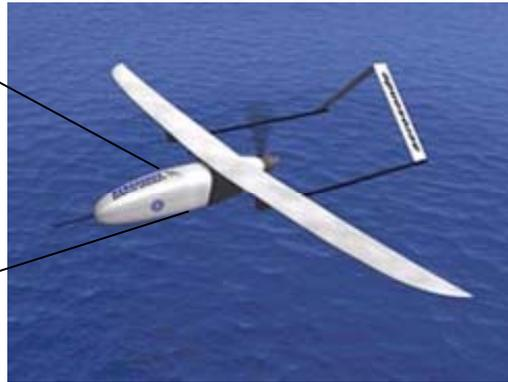
Figure 22. Modular Radiometer on board UAV
