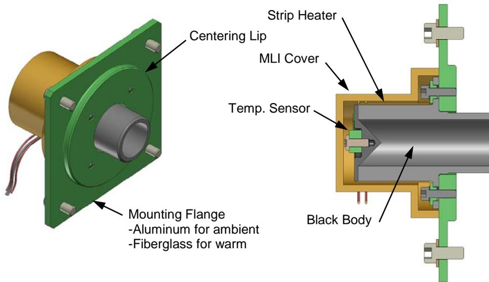
**Figure 14. Calibration Modules**
