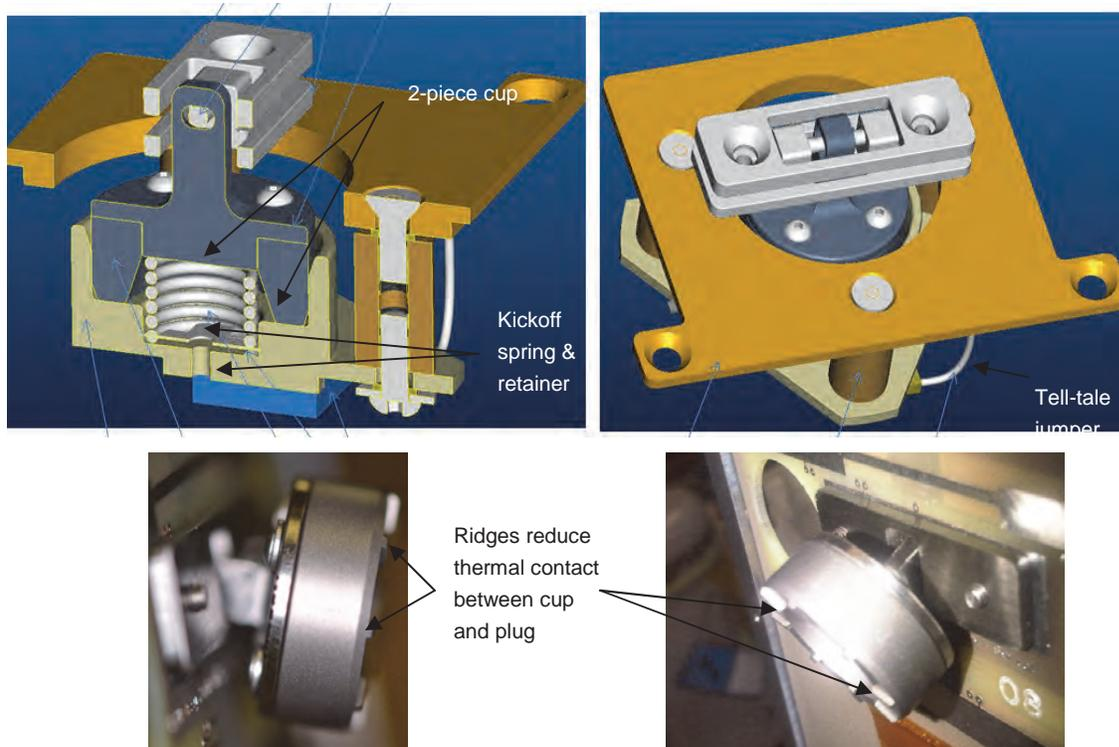
**Figure 4 – Four views of the third generation device.**
