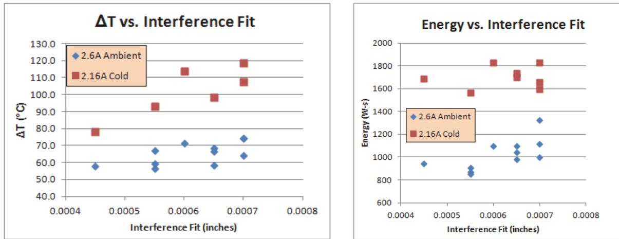
The left chart of Figure 11 shows the relationship between the initial temperature and the energy required to separate. The right chart of Figure 11 shows the relationship between actuation delta-T and the initial temperature. Since the parts were manufactured at 20°C, they will have a tighter interference fit with a lower initial temperature and will have a looser interference fit as they have a higher initial temperature.
