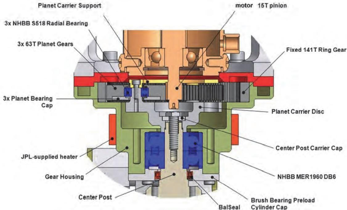
**Figure 11. Cross Section of Gearbox Assembly**
