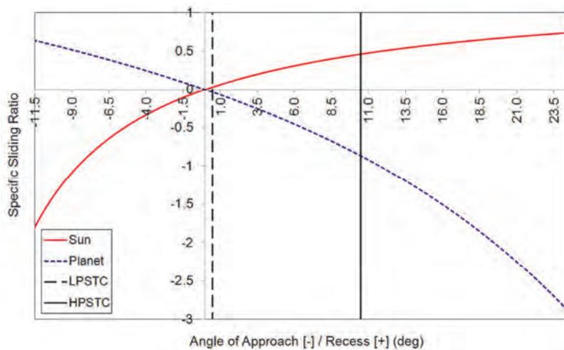
**Figure 13. Sun-planet gear mesh specific sliding ratio**
