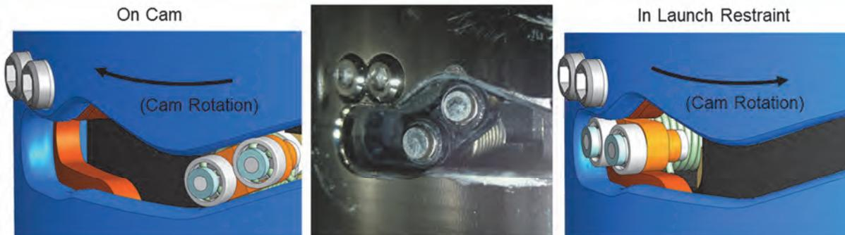
**Figure 7: Launch Restraint for Cam Follower**
