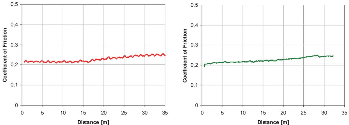
**Figure 11. Coefficient of friction versus sliding distance for Ti6Al4V pin with TiN layer and Vespel SP1 disk for vacuum environment: room temperature (left), very low temperature (right)**
