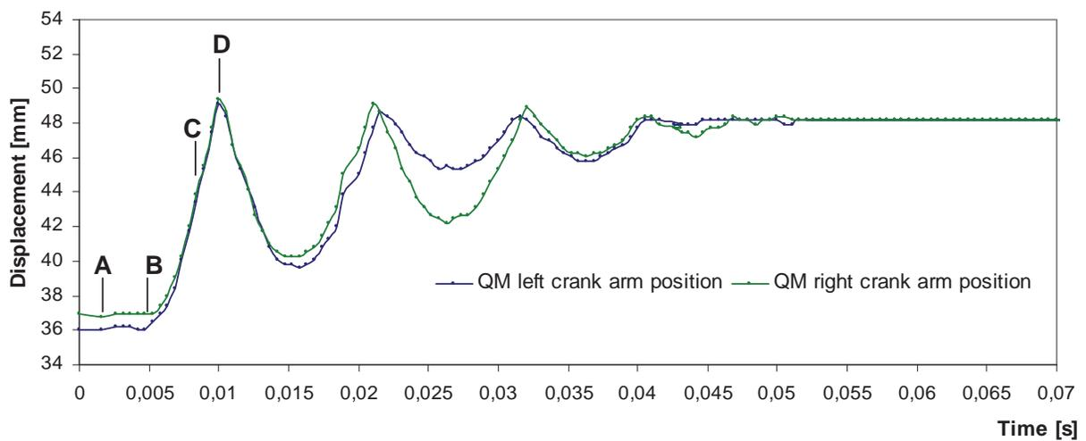
**Figure 7. Holding pins displacement during mechanism release**
