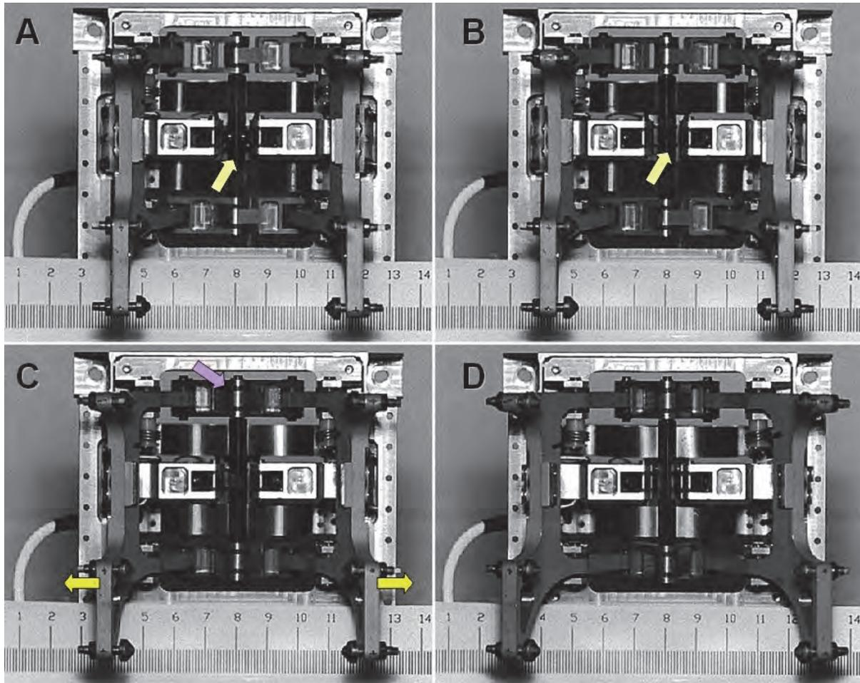
**Figure 8. Lock & release mechanism action - penetrator is removed**
