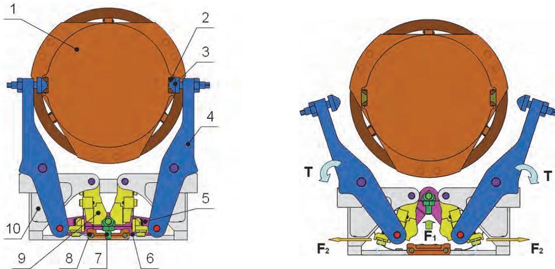
1 - PENETRATOR    2 - SOCKETS    3 - HOLDING PINS    4 - CRANK ARMS    5 - BINARY LINKS
