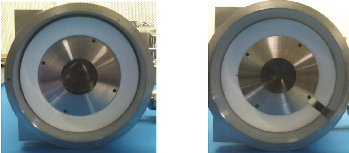
**Figure 13. Solid and Slotted designs of the guide on Test Mandrel and inside the Test Housing with the largest possible radial clearance. Note that the slotted design springs outward, closing the radial clearance under all conditions.
