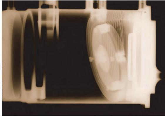
**Figure 6. X-ray of Accumulator Assembly showing bellows shape with the maximum allowable pressure difference across the bellows. The accumulator fluid capacity is significantly reduced from the required value.**
