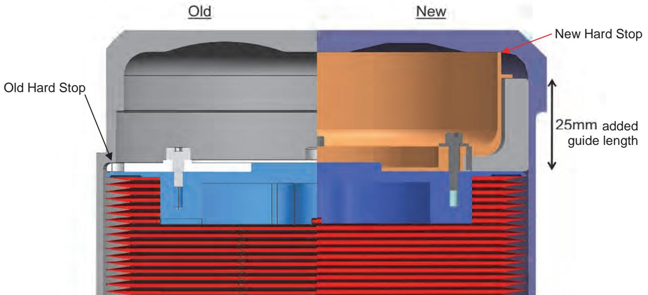
**Figure 14. Original and Final designs of the end of the bellows assembly. The figure shows the bellows stroked to the maximum fluid condition and against the end-of-stroke hard stop for both design versions**
