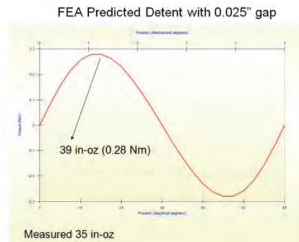
**Figure 3. Initial T Motor Detent Analysis and Measurement**
