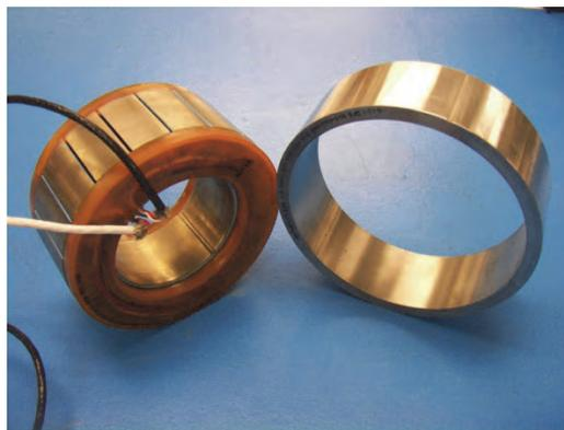
**Figure 13. Photo of the G Motor - Rotor is encapsulated in titanium ring**
