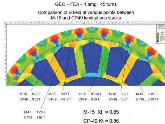
**Figure 10. Flux Density Comparison of Lamination Materials**
