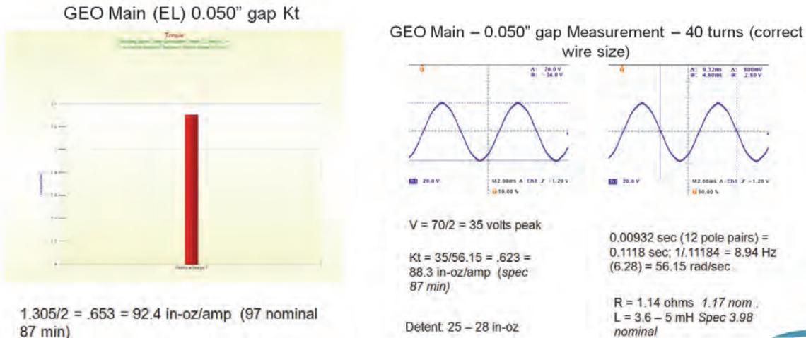
Figure 8. Motor with 1.27-mm (0.050-inch) air gap
