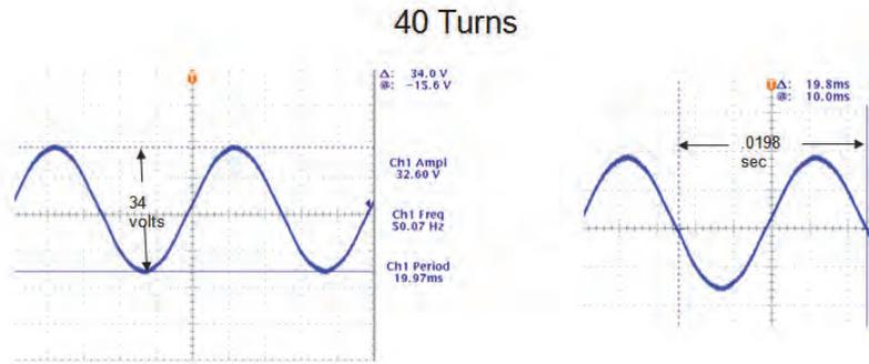
**Figure 16. BEMF for H motor with M-15 Material**
