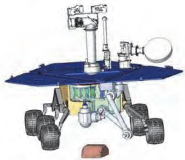
**Figure 3. Bit change-out and sample transfer configuration**
