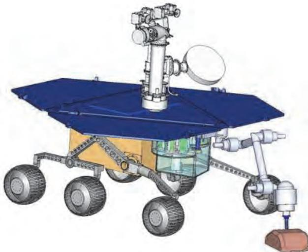
**Figure 2. IMSAH coring tool deployment**
