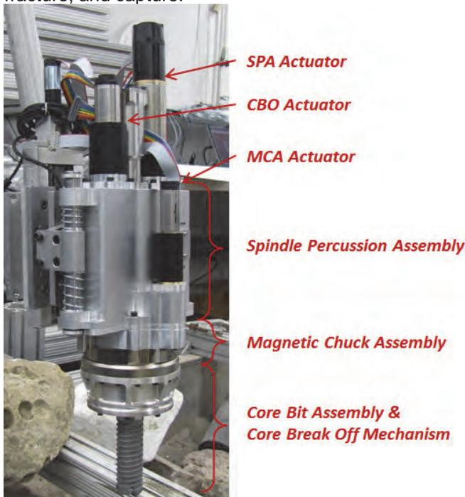
**Figure 5. Rotary Percussive Sample Acquisition Tool (SAT)**
