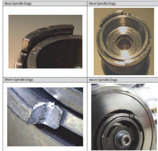
Figure 12. Accelerated wear at torque couplings
