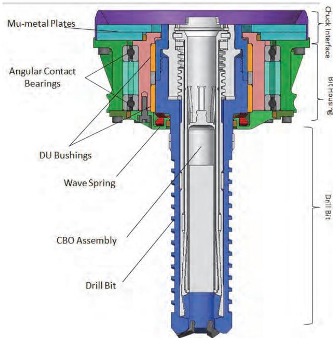
Figure 14. General schematic of the CBA
