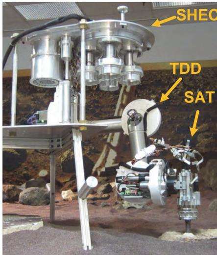
**Figure 1. Integrated sample acquisition and caching prototype subsystem.**
