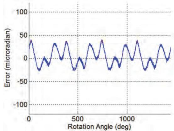
Figure 18. Synchronous Error Versus Angle
