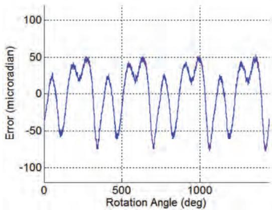
Figure 17. Synchronous Error Versus Angle
