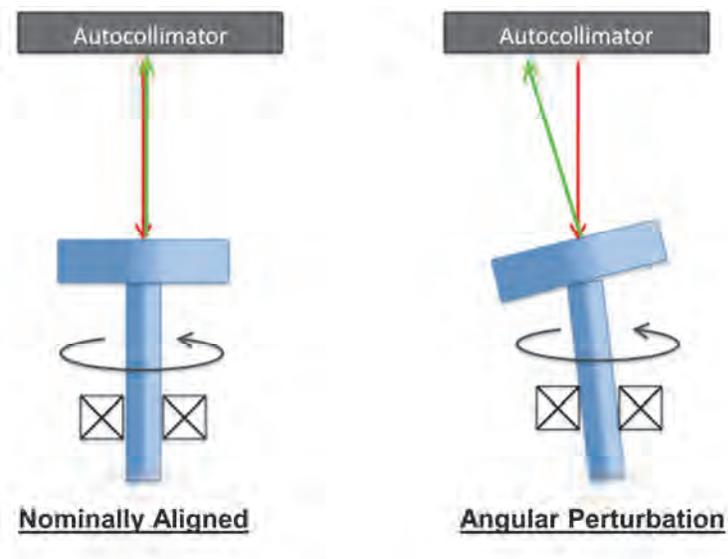
**Figure 3. Measurement Method Overview**
