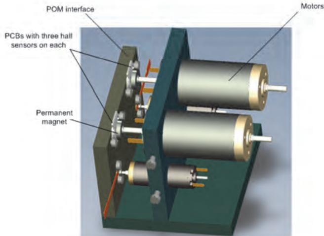
**Figure 14: Test setup for hall sensor irradiation with test configuration of 4 PCBs, each with 3 hall sensors of one type, mounted in front of four motors with permanent magnets attached to their output shafts.**
