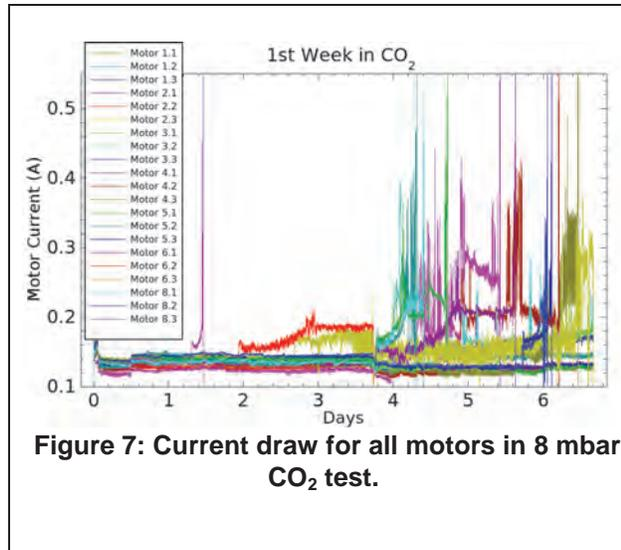
**Figure 7: Current draw for all motors in 8 mbar CO<sub>2</sub> test.**
