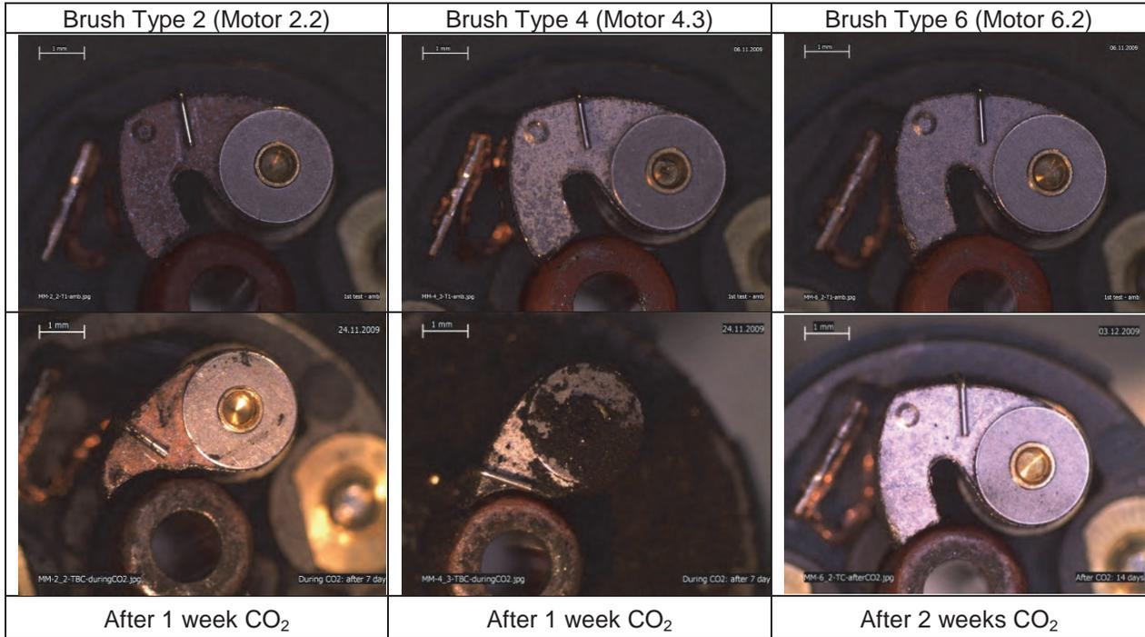
**Figure 11: Pictures of the RE13 brushes after 1 week operation in Earth atmospheric conditions (top row) and 1 week operation (2 weeks for type 6) in an 8 mbar CO<sub>2</sub> atmosphere (bottom row).**
