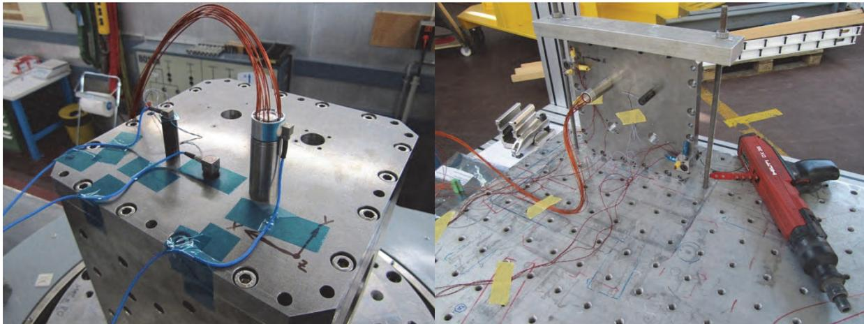
**Figure 16: Picture of RE13 & EC22 test motors attached to a stiff mounting cube (note the feedback accelerometers attached to both motors in the left picture) on the shaker (left) and on a plate for the shock test (right). The powder actuated nail gun used to impart the shock is visible at the right.**
