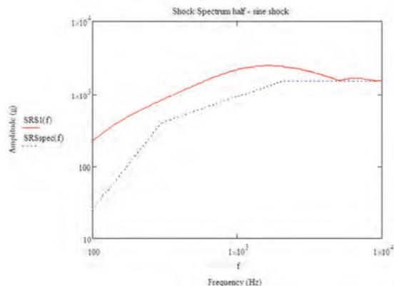
**Figure 5: Shock response spectrum applied on the motors**
