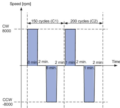
Figure 18: Reference cycle for RE13
