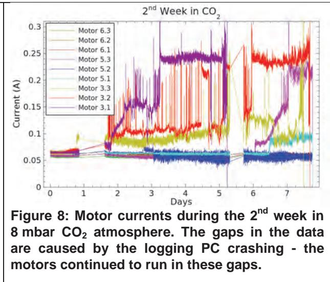
**Figure 8: Motor currents during the 2<sup>nd</sup> week in 8 mbar CO<sub>2</sub> atmosphere. The gaps in the data are caused by the logging PC crashing - the motors continued to run in these gaps.**
