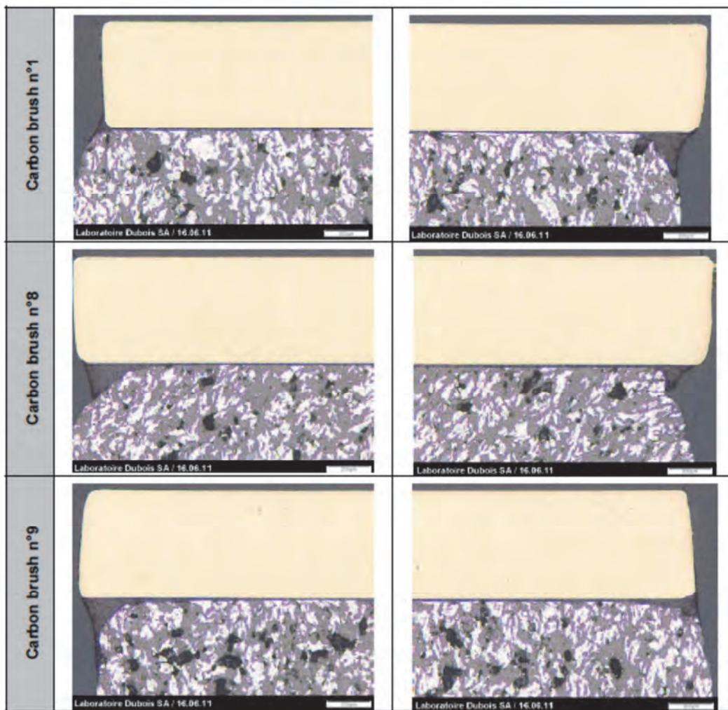
Figure 4. Example of composite brush micro-section views (© Laboratoire Dubois SA)
