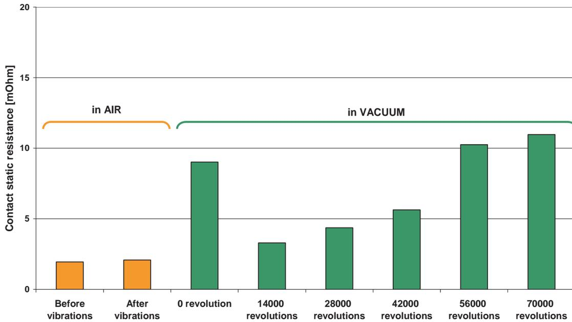
Figure 8. Static contact resistance evolution – RMS value
