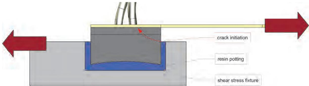
Figure 3. Shear test setup and fracture mode description
