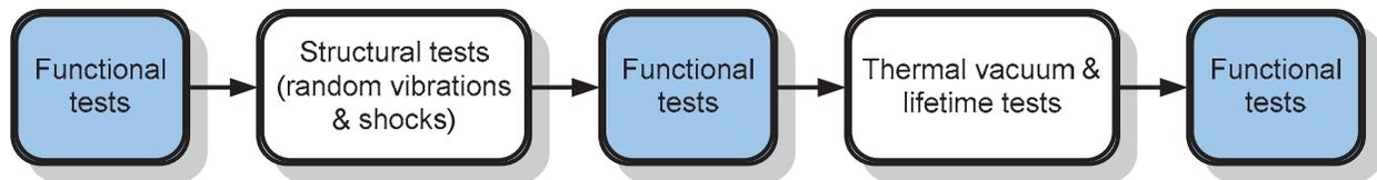
**Figure 7. Breadboard models validation sequence**
