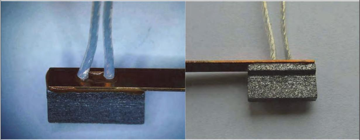
Figure 16. Close-up view of glued interfaces
