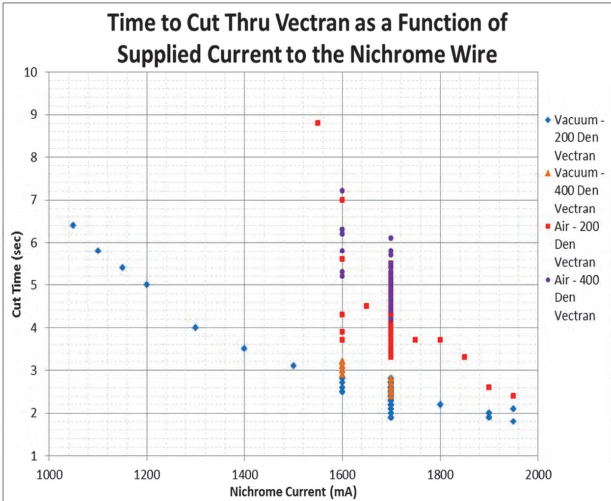
demonstrated that when using the tight tolerance constant current circuit the burn wire release mechanism can be actuated at least 50 times without having to change out the nichrome wire. Many of the burn wire release mechanisms were used past the 50 actuations, up to 80 actuations, and still performed nominally Figure 7 shows the release mechanism immediately following a successful cut through the Vectran cable in vacuum with the nichrome wire still glowing hot.
