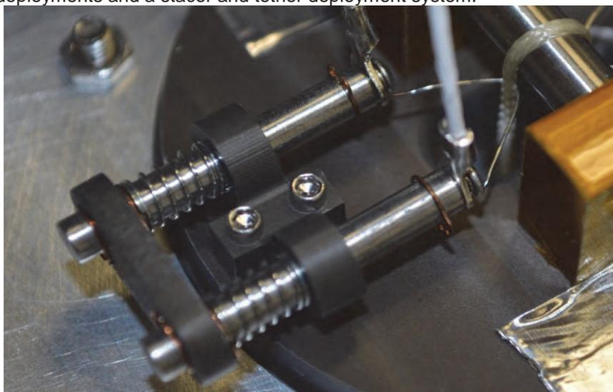
Figure 1. Assembled burn wire release mechanism
