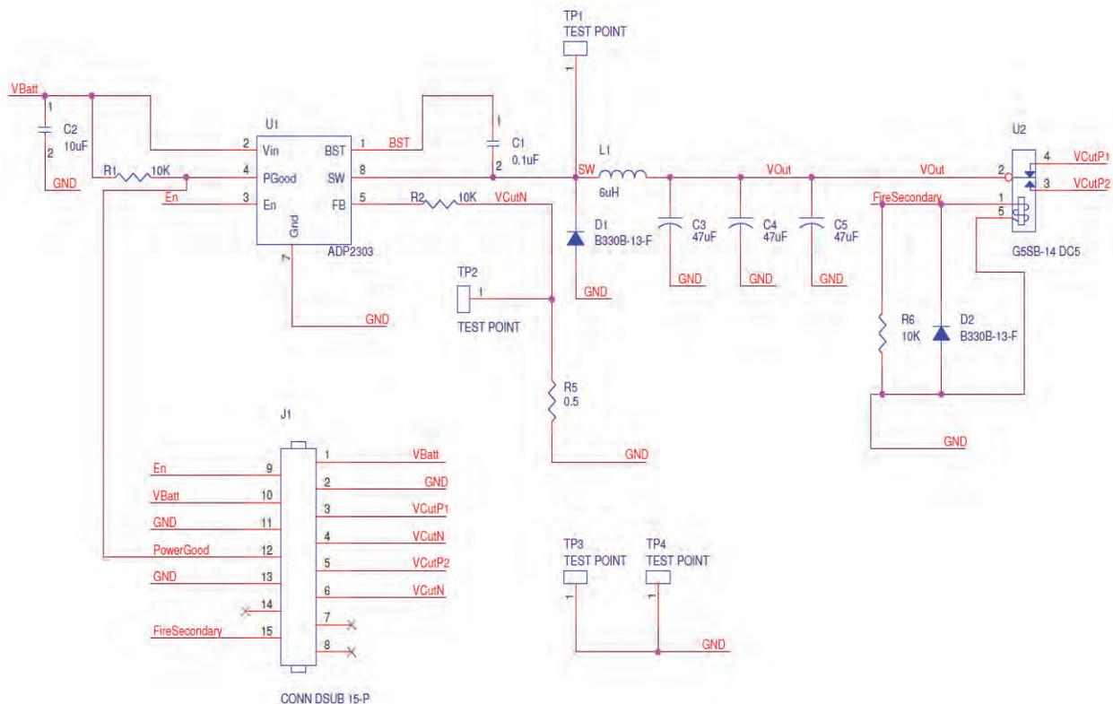
Figure 5. Schematic for the constant current circuit design.
