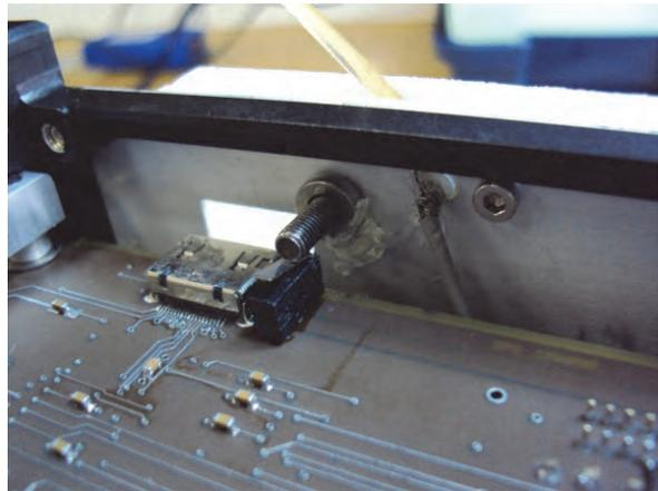
Figure 14. PEM nut for guiding the RBF
