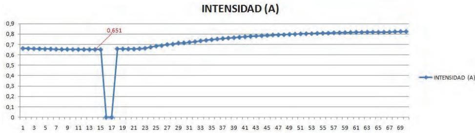
**Figure 6. Monitored intensity during burning thermo-vacuum test**
