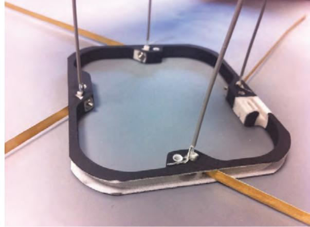
**Figure 16. Coated Sub-chassis during the integration process**
