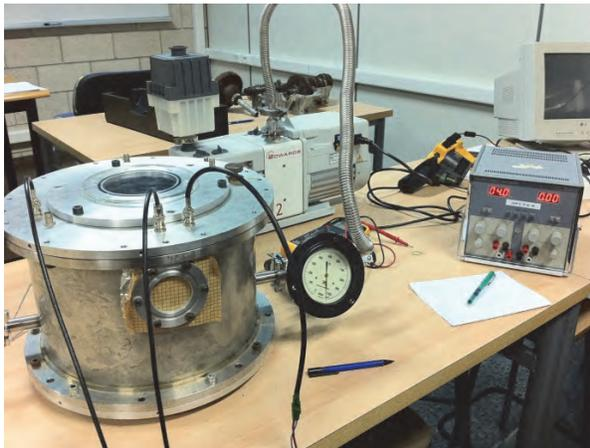
Figure 4. Thermo-vacuum chamber
