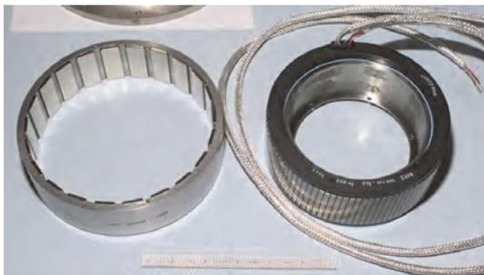
**Figure 7. BAPTA 3-Phase DC torque motor**
