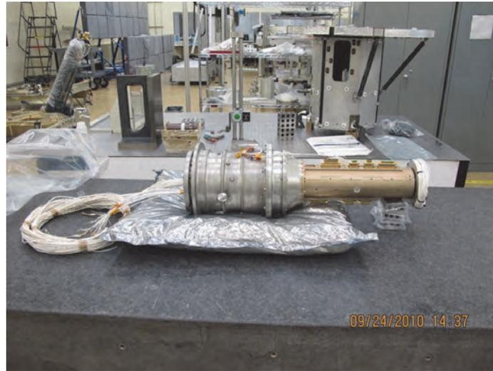
**Figure 1. The completed Flight 1 SMA Assembly**
