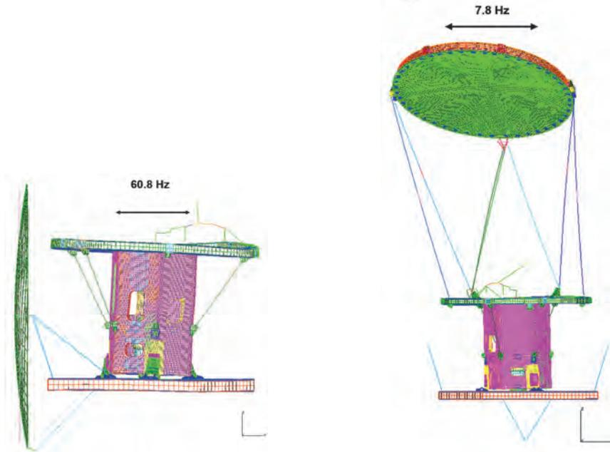
**Figure 4. Finite Element (FEM) model of GMI instrument with SMA and launch restraints meets the first mode stowed frequency requirement (>50 Hz), meets the first mode minimum deployed frequency requirement (>6 Hz) predicted on-orbit**
