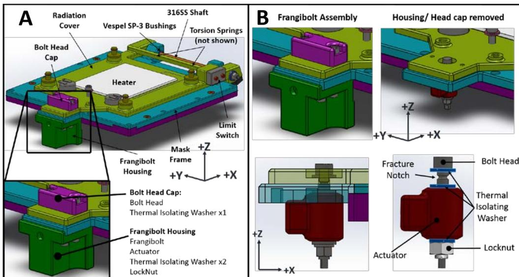
**Figure 1. (a) The REXIS radiation cover in closed configuration (b) detail of the Frangibolt assembly**
