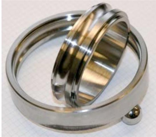
**Figure 5. 60NiTi Bearing Races.**
