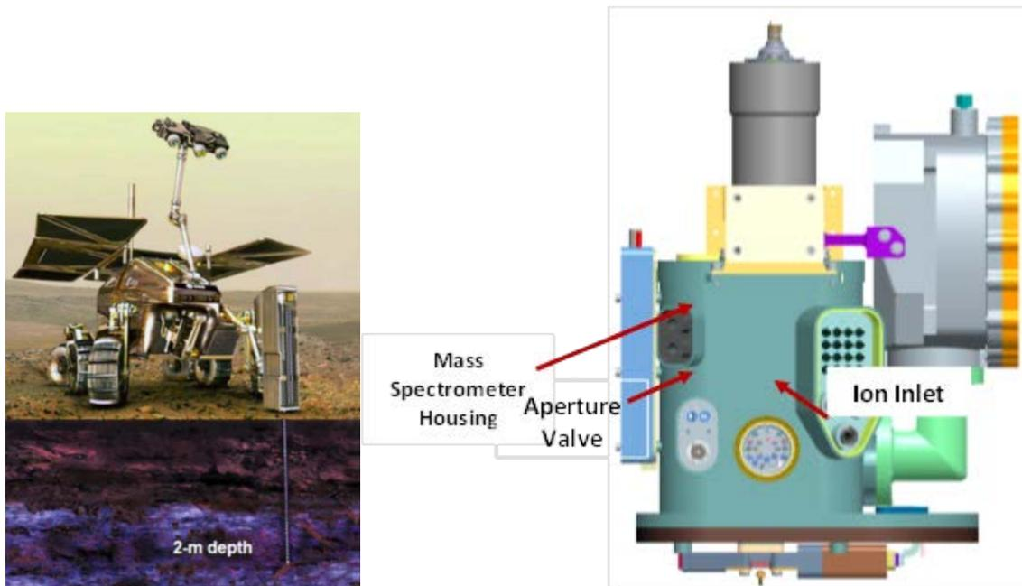
**Figure 1. MOMA Mass Spectrometer with Aperture Valve**
