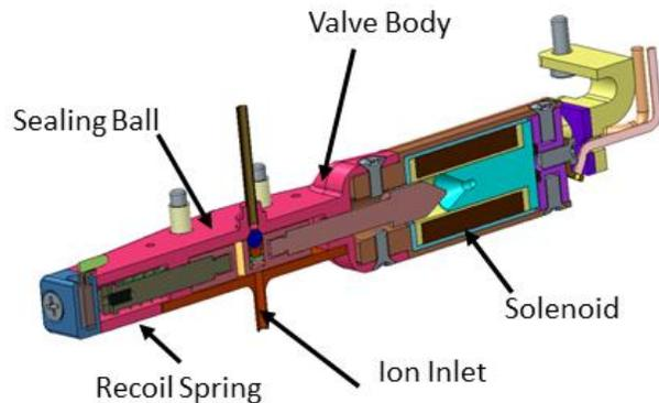
**Figure 6a. ETU /Flight Valve Section**
