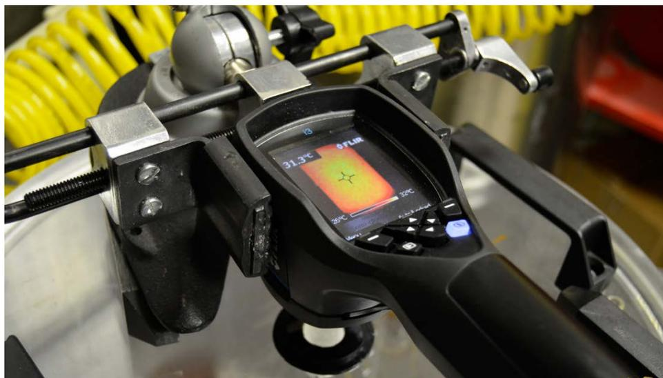
**Figure 4. Thermographic (FLIR) instrument positioned above CaF<sub>2</sub> port in top of chamber.**
