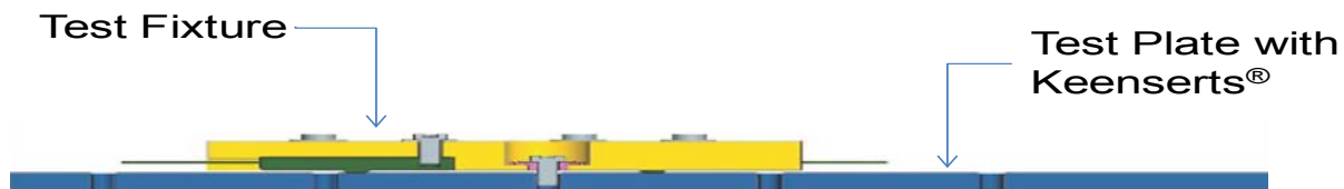
Figure 1. Bolt Preload Test Fixture & Test Plate
