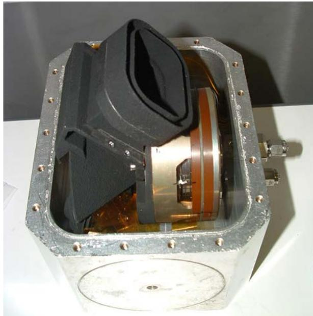
**Figure 9. PACS FW in the sealed vibration adapter**
