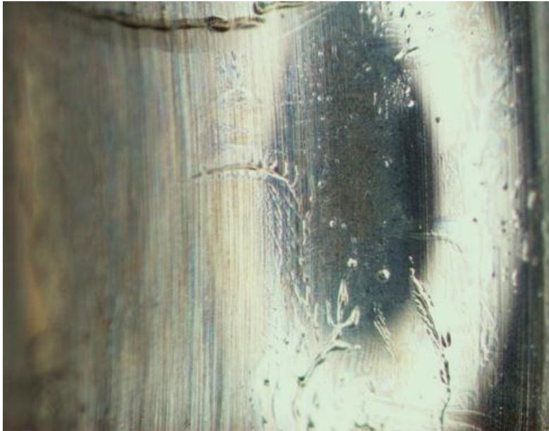
**Figure 8. A higher magnification view of the race in Figure 7, clearly showing the worn off hone lines and darkened grease in upper portion of the photomicrograph.**
