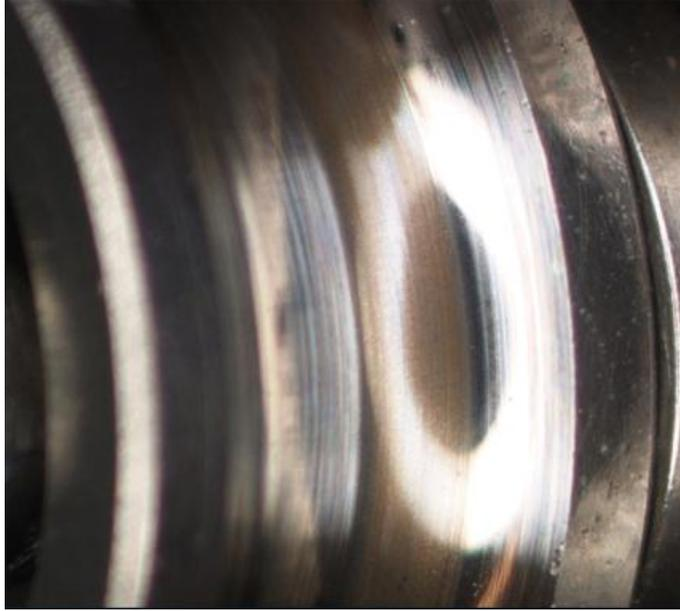
**Figure 6. 6-mm (0.2-in) race that generated the data shown in Figure 3, oil - only test. Note the worn ball path where hone lines have been eliminated when all-steel balls and rings/races are used.**
