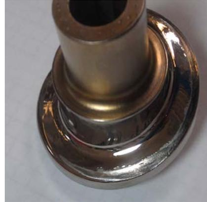
**Figure 12. Wear on SASSI CAM**
