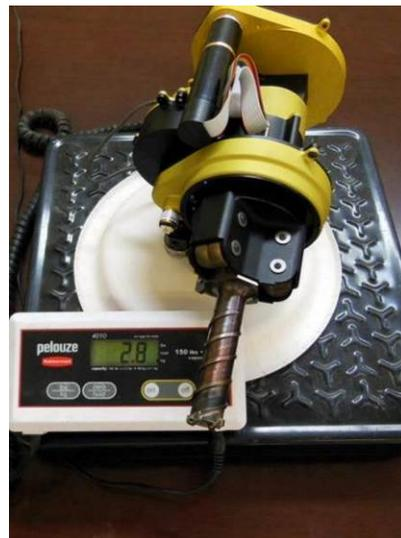
**Figure 1. Weigh-in picture of the final mechanical assembly of the RANCOR drill**
