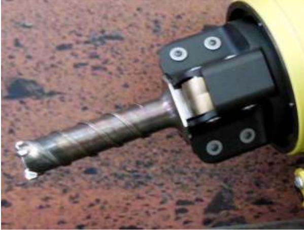
**Figure 7. RANCOR drill chuck and drill bit**
