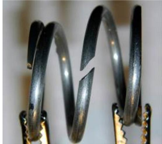
**Figure 17. Post failure spring, side 1 on the left, side 2 on the right. An approximate 45 degree failure to the surface of the spring corresponds with the maximum principal stress plane.**
