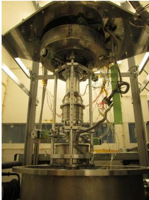
**Figure 5. 1:21 Magdrive Cryogenic prototype with superconducting bearing and test bench. A perfectly cryogenic non-contact Magdrive. Max. torque 4 N-m, max speed 1500 rpm at 50-90 K. Weight 7.5 kg. Envelope 130-mm diameter. Length 600 mm.**
