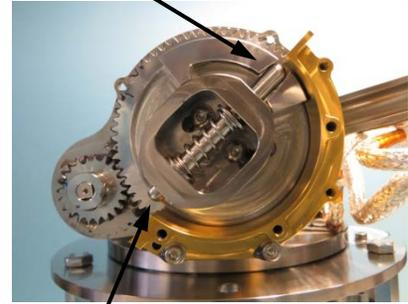
pin is no longer constrained by housing, hinge shaft is free to rotate
