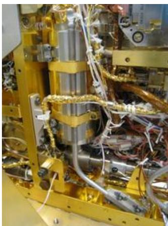
**Figure 4. Wide Range Pump Installed in SAM Instrument**
