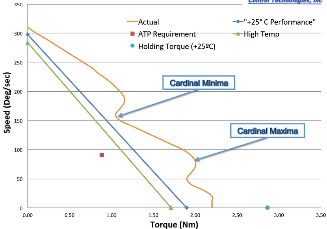
Figure 2. Empirical Dynamic Performance versus Linear Simulation
