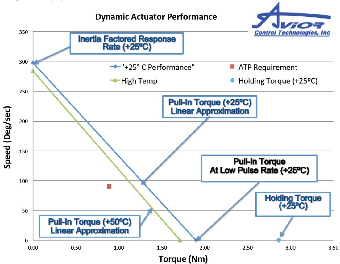
**Figure 1. Linear Simulation of Geared Stepper Motor**
