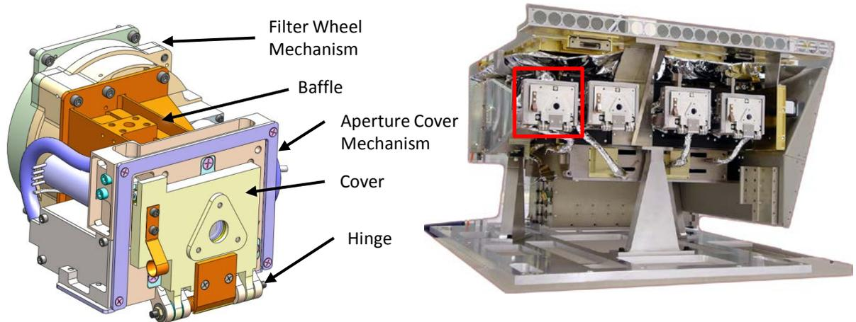
**Figure 1. SDO/EVE Aperture assembly with four aperture cover mechanisms**
