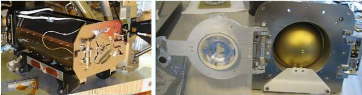
**Figure 2. MMS/SDP Sensor Restraint Mechanism**
