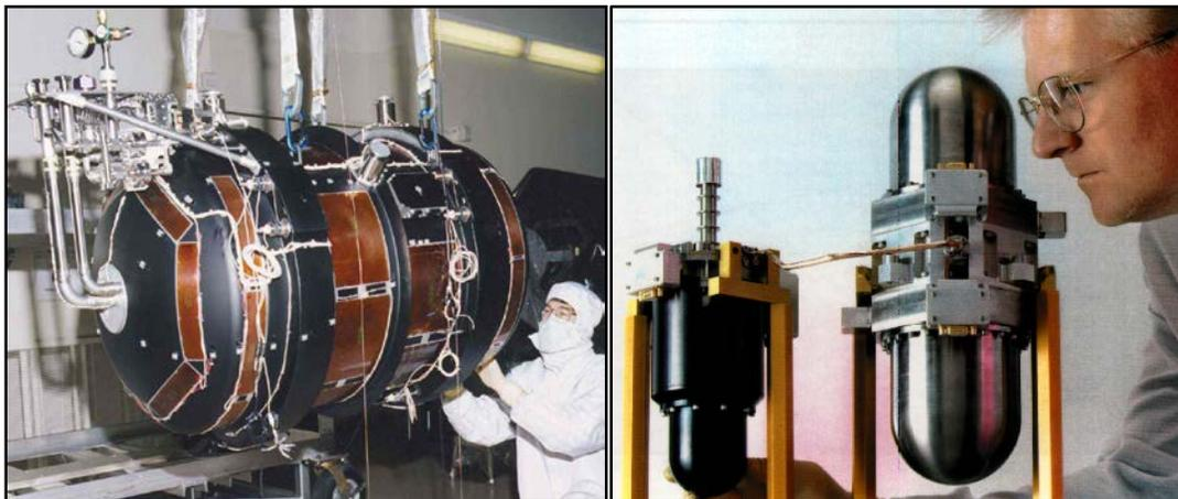
**Figure 6. Early expendable cryostats (left) and cryocoolers (right)**
