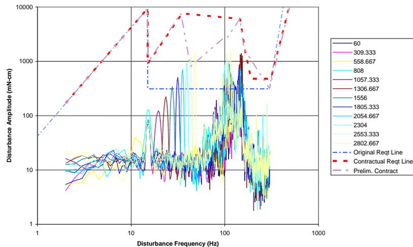
Figure 2.4: X-axis disturbance torquespeeds in RPM.
