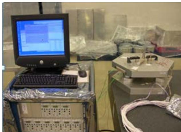
Figure 3. An Integrated example of a model of a mechanism with a later generation of BATC FMP (left) and 1 KHz FMP, charge amplifiers and computer system for data acquisition (right)
