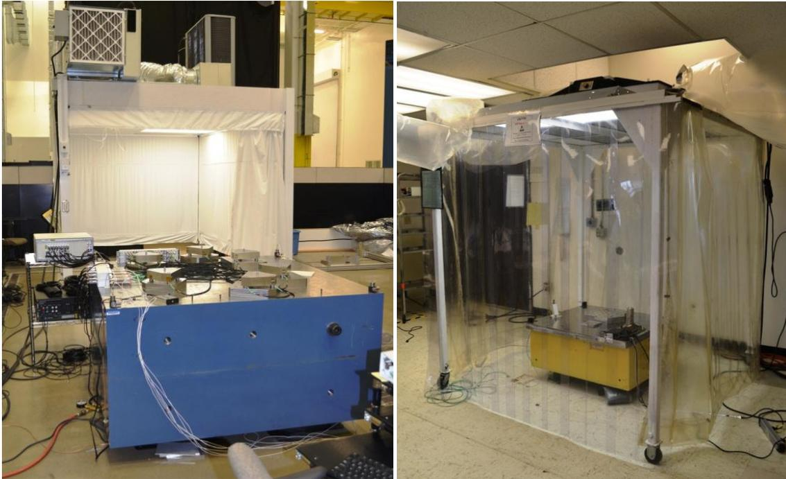
**Figure 1. EFT tables with clean tents: 30,000 lb (60" x 60") (left) and 4,400 lb (36" x 34") (right) 133 kN (1.5 m x 1.5 m) (left) & 19.6 kN (.91 m x .86 m) (right)**
