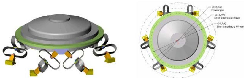
Figure 9. BATC Robi Wheel on jitter isolation mount
