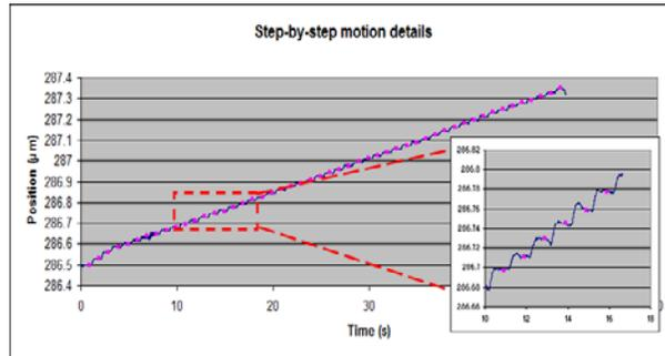
**Figure 9. Motor displacement and resolution (mean step = 20 nm)**
