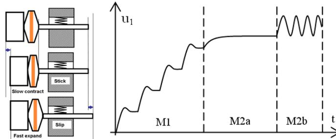
**Figure 4. SPA components and principle: stepping mode (M1) and deformation mode (M2)**
