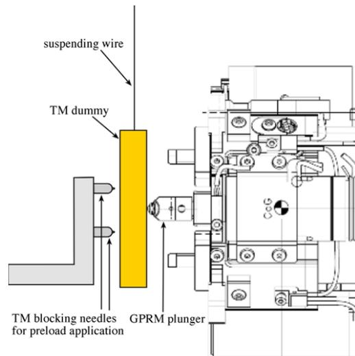
**Figure 9. Test configuration with GPRM EQM -Z**
