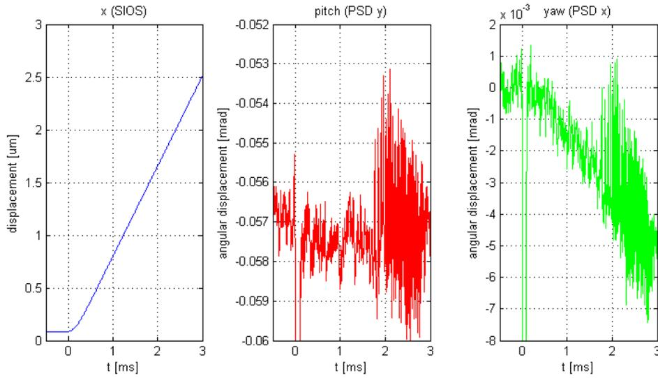
**Figure 12. TM displacement, pitch and yaw signals**
