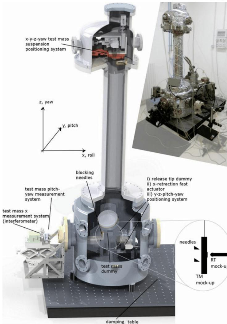
**Figure 3. The Transferred Momentum Measurement Facility**
