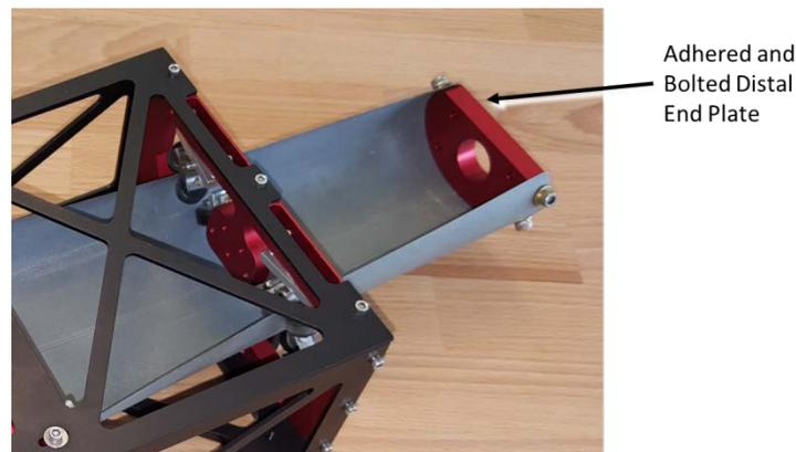
**Figure 6. 'NASA ARM Boom' Deployer, Distal End**
