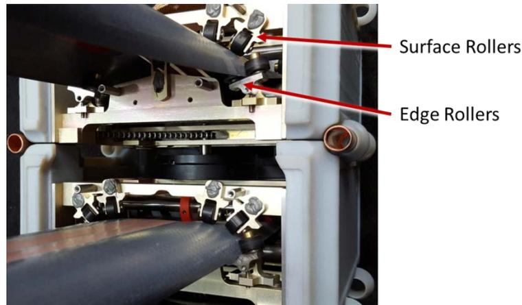
**Figure 7. 'DARPA Phoenix HIMast Boom' Boundary Condition Restraints**
