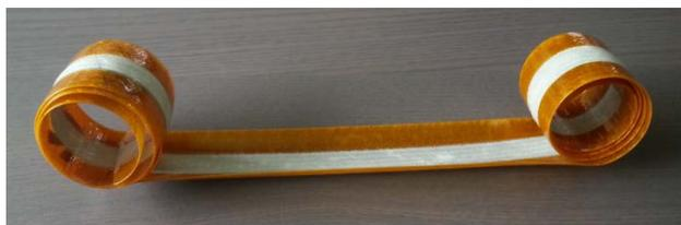
**Figure 4. Example of a Neutrally Stable Boom (Glass Fibers)**
