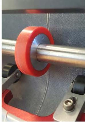
**Figure 9. 'NASA ARM Boom' Deployer Drive Wheel**
