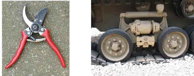
**Figure 2. Terrestrial uses for volute springs**
