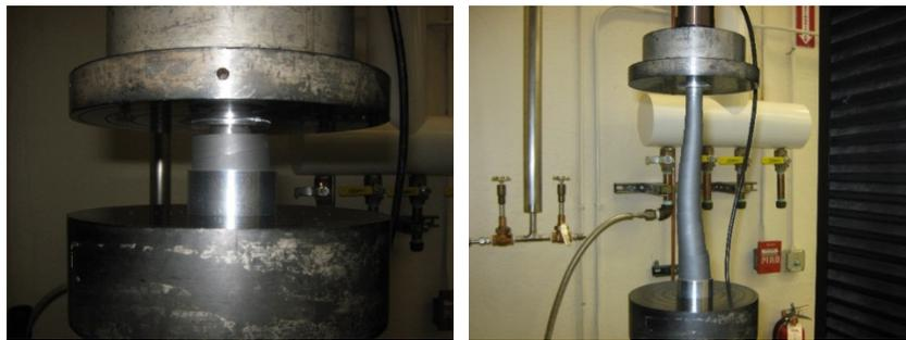
Figure 6. Instron Test Fixture for Load vs. Deflection Curves
