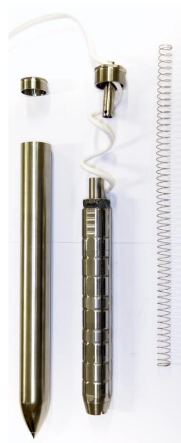
**Figure 5. Outer casing, driving sections and return spring just before final assemblage.**
