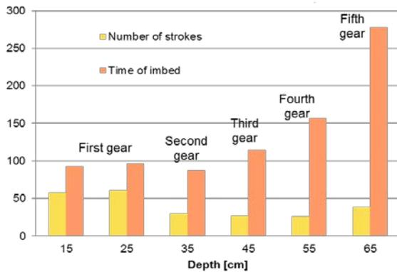
**Figure 8. Dependence of number of strokes and time of imbed from depth for five power settings.**
