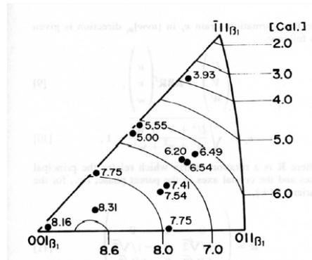
**Figure 2. Relation between transformation strains and crystal orientation <sup>(3)</sup>**
