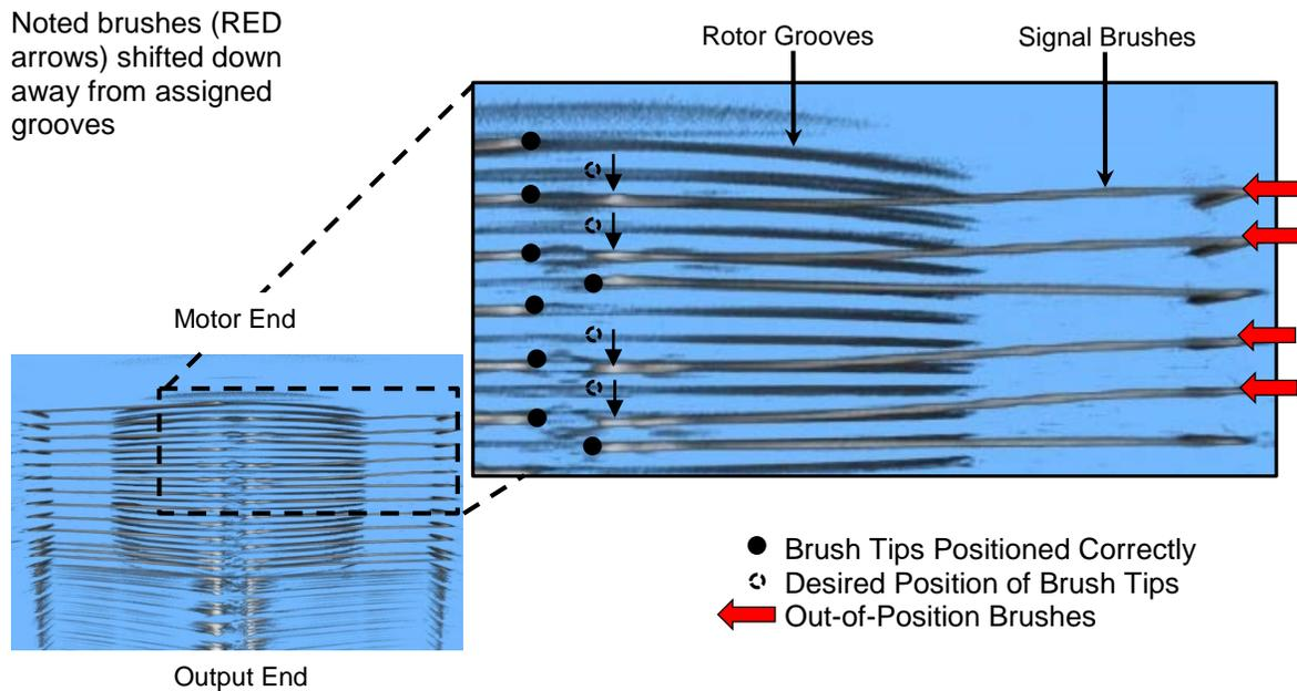
**Figure 6. Radiographic Image of SADA Slip Ring with 4 Shorted Signal Brushes**
