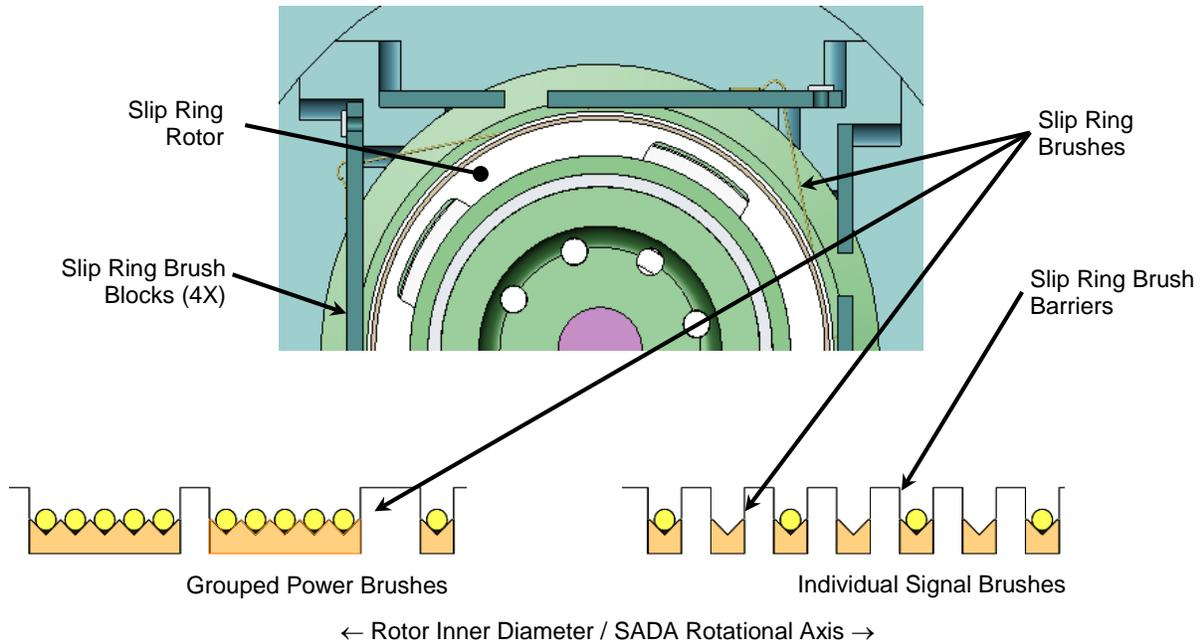
**Figure 5. Illustration Slip Ring Rotor Ring Grooves and Brush Orientation**
