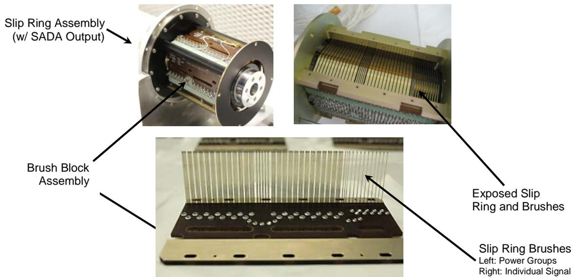
**Figure 4. Slip Ring Assembly w/ Exposed Rotor and Brushes**
