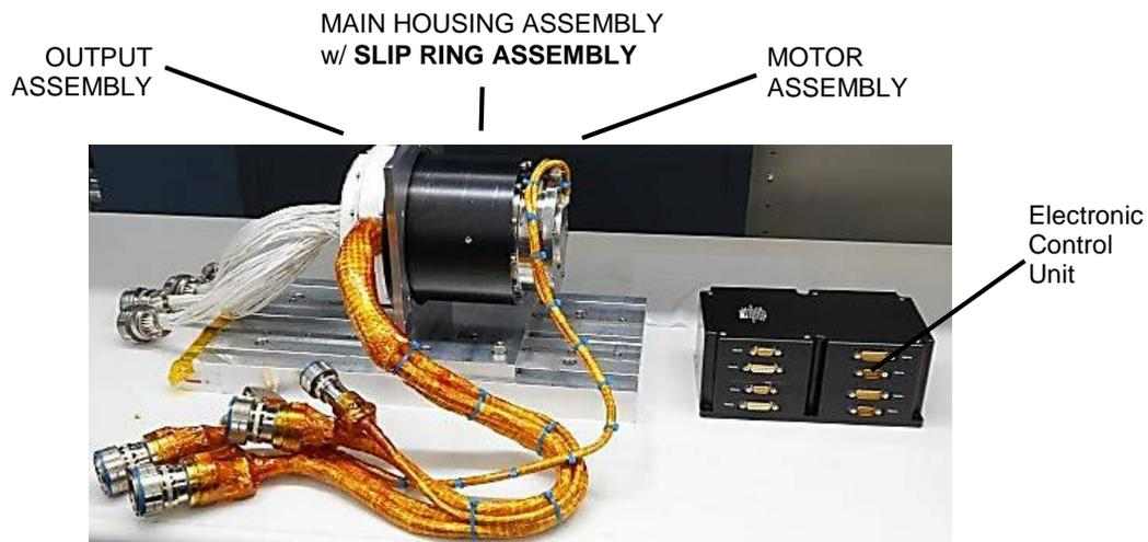
**Figure 1. SADA System w/ Electronic Control Unit**
