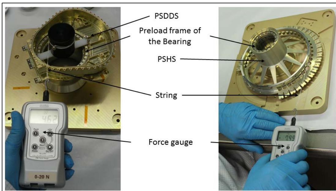
**Figure 6. Test setup to measure the preload torque**
