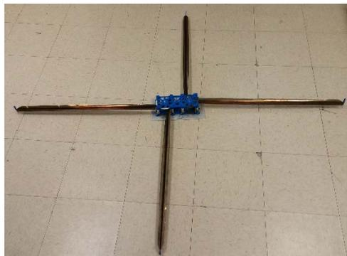
**Figure 10. Boom Deployer Prototype with flight-like TRAC booms**
