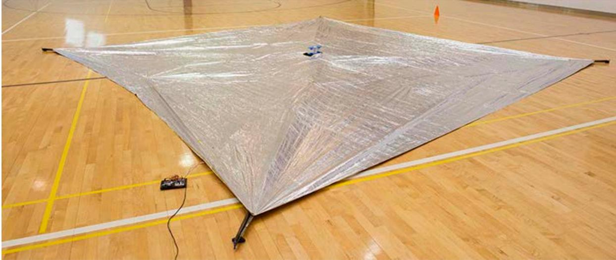
**Figure 23. Deployed Solar Sail After Second Deployment**
