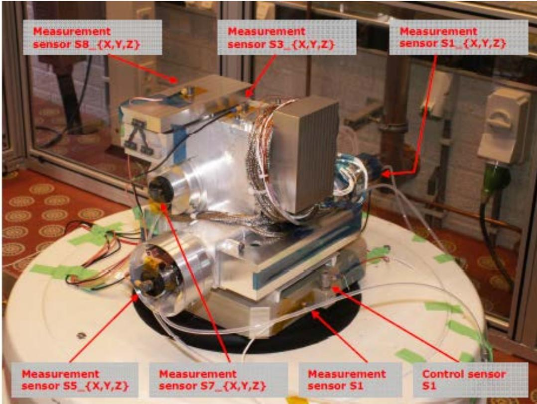
Figure 11. Vibration testing of the CU with a 9.71 g<sub>rms</sub> input spectrum, resulting in 28.6 g<sub>rms</sub> on the carousel
