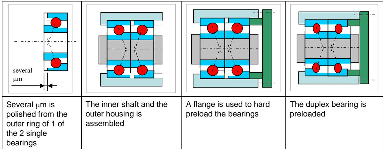
**Figure 2. The principle of a duplex bearing**
