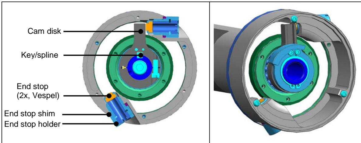
**Figure 8. The FMM is equipped with an end stop in order to guaranty an angular reproducibility < 0.1°. A cam disk will rest on an adjustable Vespel end stop. Note that two stops are incorporated.**
