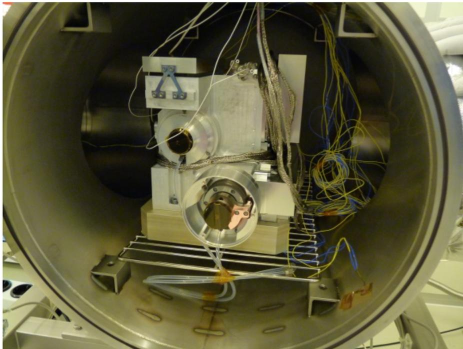
Figure 12. Thermal Vacuum Testing of the CU
