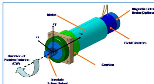
Figure 1. JWST Deployment Brushless DC Geared Motor Overview
